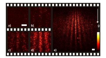
The molecules used in this experiment have an atomic mass of 1298 amu (2.15 x  $10^{-24}$  kg). In order to detect the very small wavelength, the molecules needed to be travelling very slow. The molecules were found to have an approximate wavelength of 5.20 pm.
